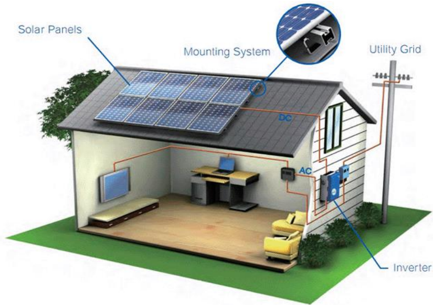
Figure 5. On-grid residential photovoltaic systems.
