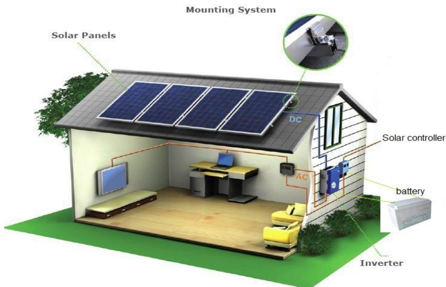
Figure 6. Off-grid residential photovoltaic systems.
