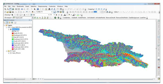
**Figure 2.** The exposure map of the slopes of Georgia. The image legend indicates conditional signs of the slope exposure by colour: N exposure is shown in red, NE - in orange, E - in light green, SE - in green, S- in blue, SW - in light blue, W - in yellow Blue, SW - with violet.
