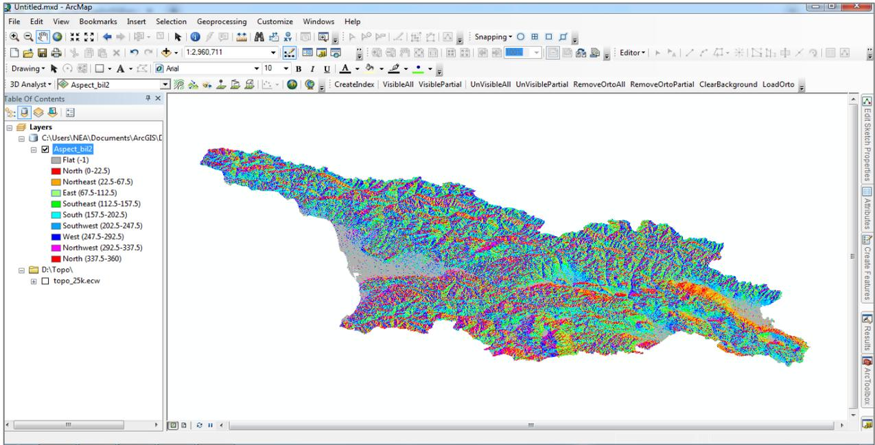
**Figure 2.** The exposure map of the slopes of Georgia. The image legend indicates conditional signs of the slope exposure by colour: N exposure is shown in red, NE - in orange, E - in light green, SE - in green, S- in blue, SW - in light blue, W - in yellow Blue, SW - with violet.
