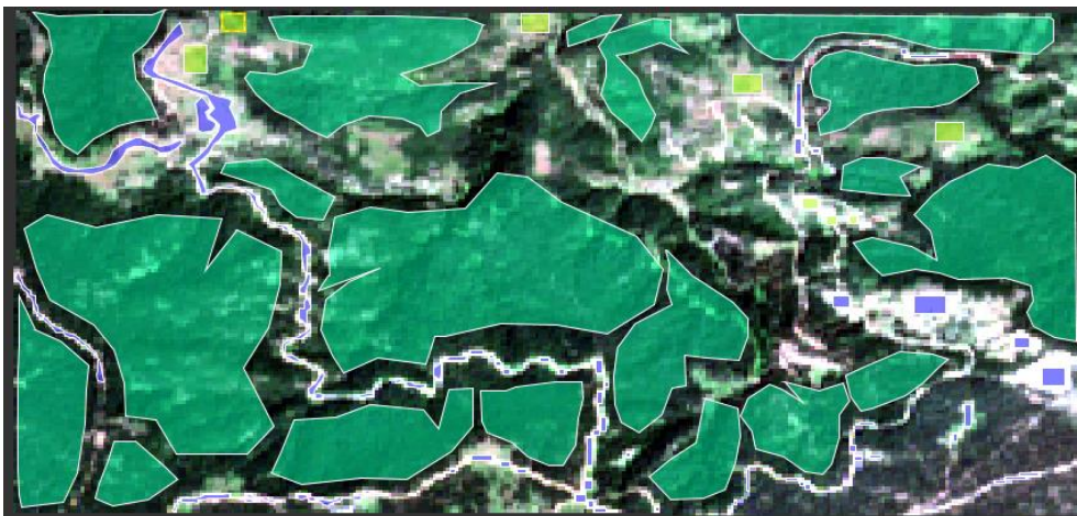
Figure 4. Controlled classification for 2023 satellite images (Green: forest area, light green: bare land, purple: forest roads).
