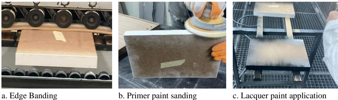
Figure 1. Preparation stages of test samples.
