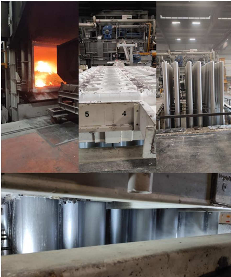
Figure 1. Production of aluminum billets by casting process.
