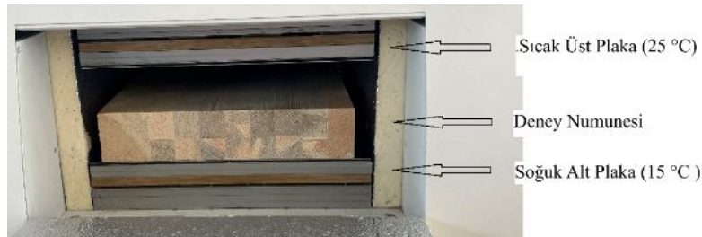
Figure 6. Test specimen in the test device.
